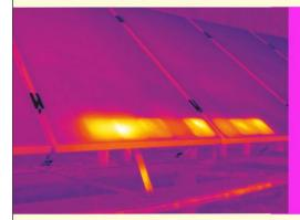
The thermal image illustrates common issues with defective cells and substrings.
