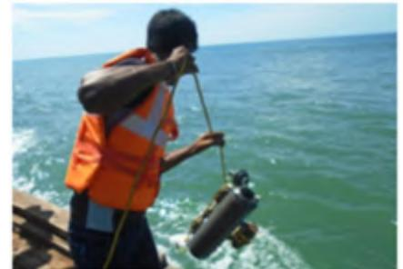
*Collection of Marine Water using Niskin Sampler*
